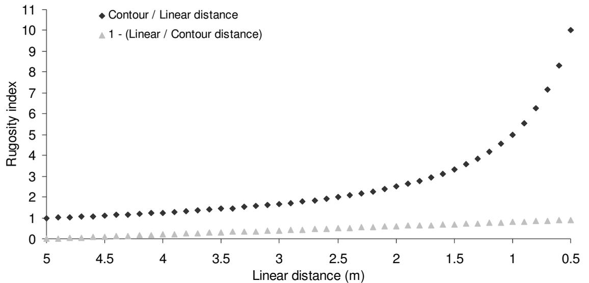
**Fig. 2.2:** Relationship between the linear distance measurement and the rugosity index using the traditional and modified formulas with a fixed contour distance of 5 metres.
